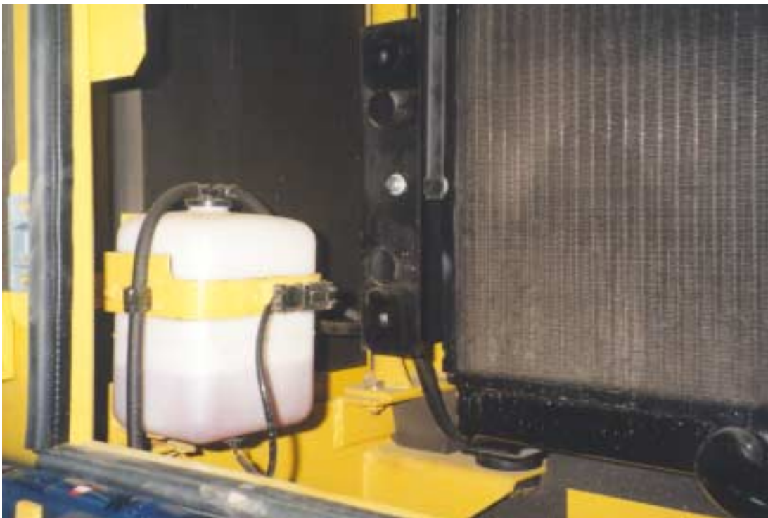
Left side lower condenser bracket with spacer behind intercooler bracket.
