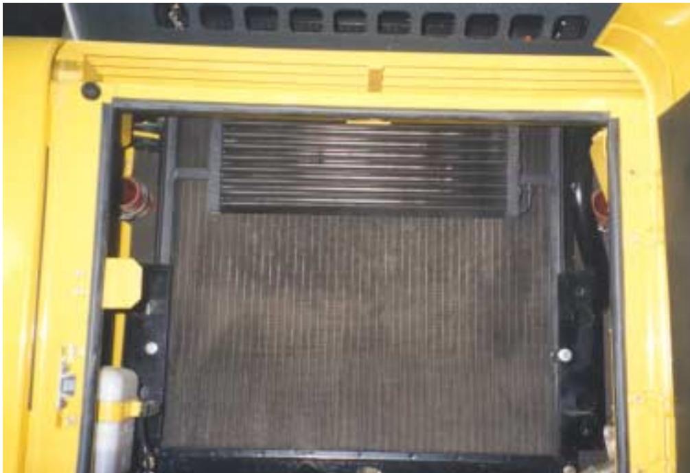
Condenser mounted in location.
