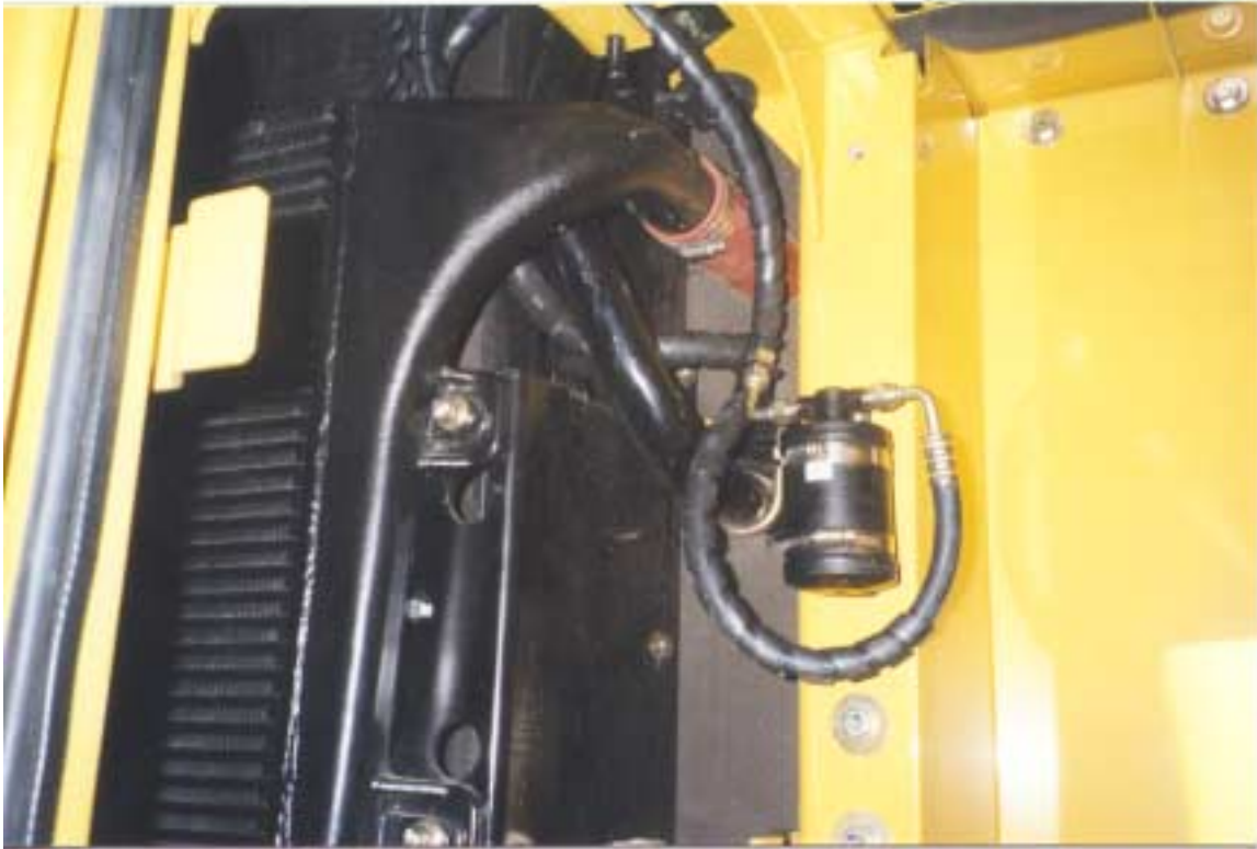
Drier mounted in place.
